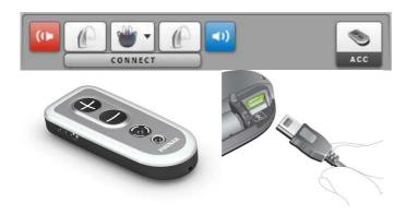
Phonak Target automatically identifies connected accessories; just plug them in during the fitting session. Always remove the battery before plugging in the USB cable. The identified accessories are shown in the dashboard next to the connected hearing instruments.
