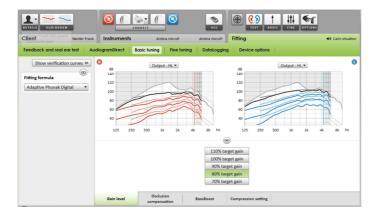
Go to [Basic tuning] if adjustments to [Gain level], [Occlusion compensation], [BassBoost] or [Compression setting] are required. The tools can be selected via the tabs in the lower part of the screen.
